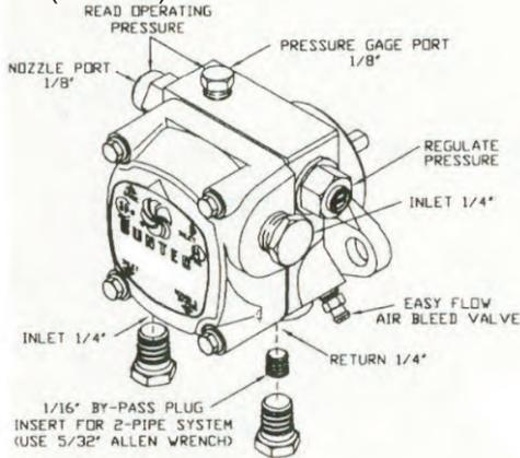
When replacing a fuel pump, ensure 1/16" by pass plug is installed in return port. Use a 5/32" allen wrench.
